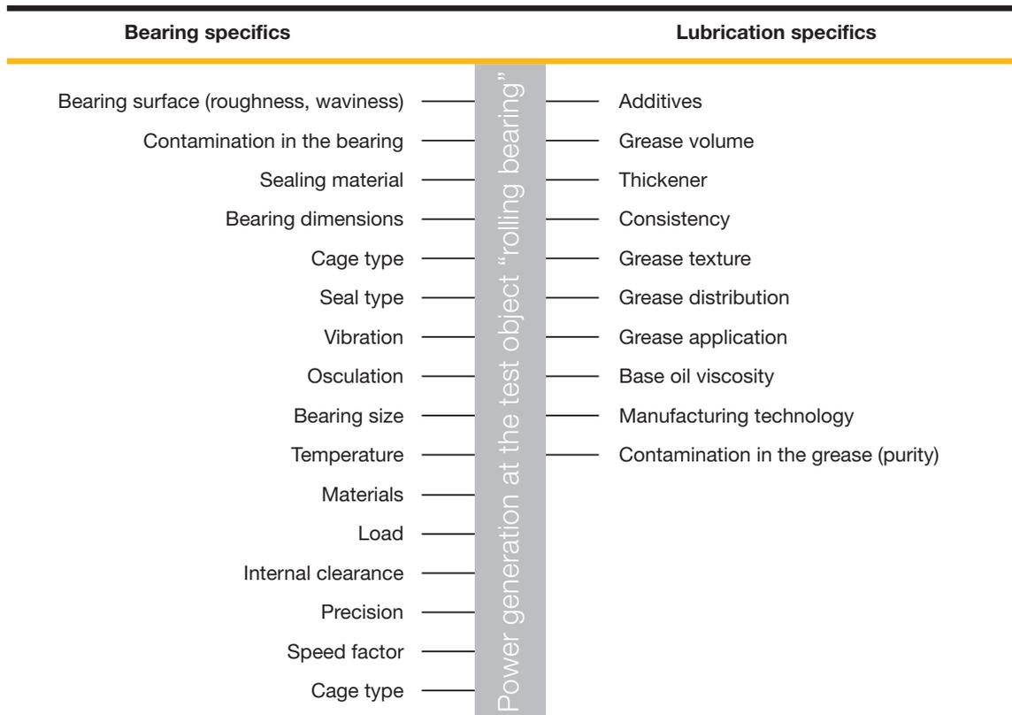
Both mechanical and lubrication-related factors can jointly influence the particular operating noise level of a rolling bearing. The combined noise behavior of the rolling bearing and lubricant is measured on special noise test equipment. It is often difficult to identify which influencing factors are responsible for generation of both solid and air-borne sound.
