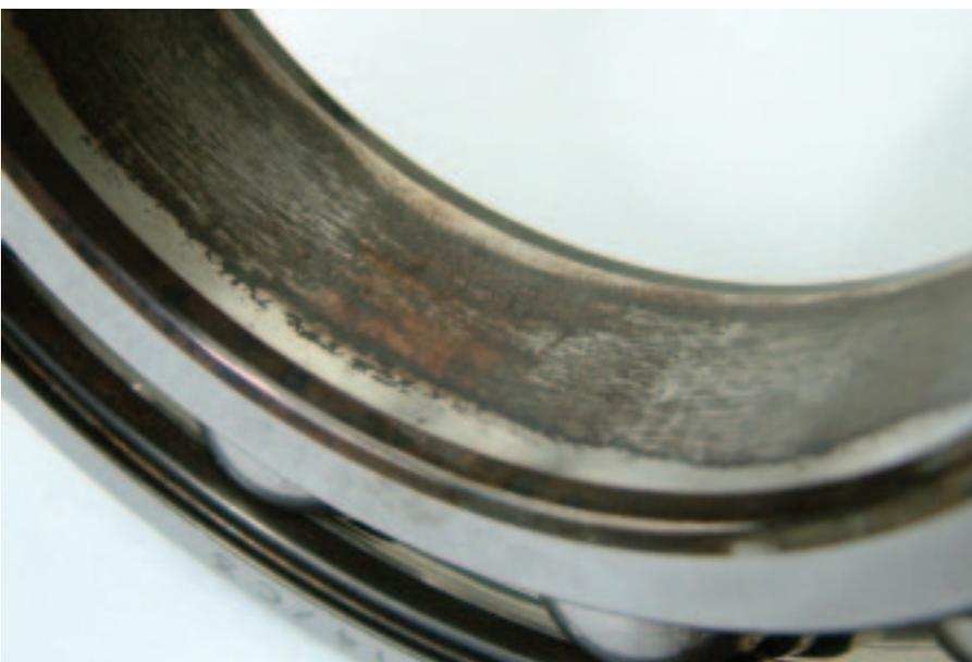
*Fretting corrosion on the inner ring*
